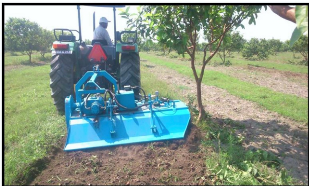
Figure 4: Working of rotary offset tiller in orchards
