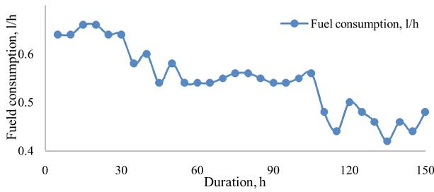
**Fig. 3: Fuel consumption of engine during the long duration test Exhaust emission**
