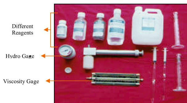
**Fig. 1: Lube oilab kit**
