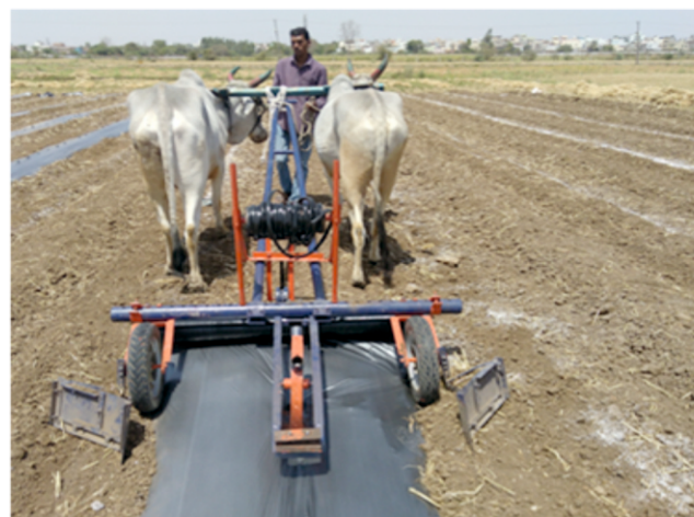
Fig. 2: Laying of mulch and drip by developed machine
