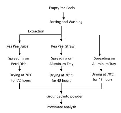
Moisture content (M) and Dry matter (DM):- Ten gram of each sample were taken in a pre-weighed petri dish/aluminum tray. The tray was placed in a hot air oven at  $70 \pm 2^{\circ}$ C for 48 hours for pea peel and peel straw, 72 hours for peel juice. The drying was repeated until a constant weight was obtained. The loss in moisture content after drying was estimated and DM was calculated as follows:
