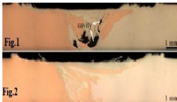
Fig.3: Influence of tool rotation speed (Fig.1)600 revolution/min and (Fig.2)1000 revolution /mint(adapted from ( Liu et al. , 2011))
