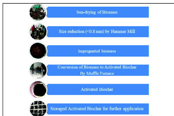
Fig. 1: Chemical activation process
