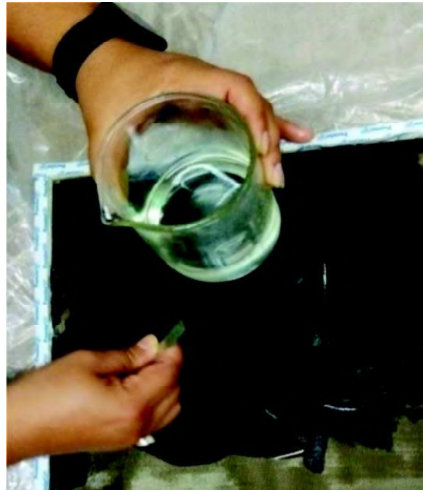
Fig.7: Initial application of epoxy resin during the hand lay-up process
