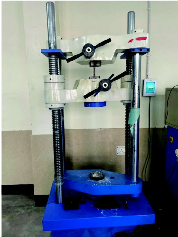
Fig.12: Universal Testing Machine (UTM) used for tensile strength measurement
