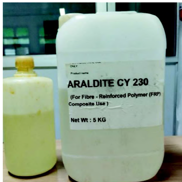
Fig.4: Epoxy resin (ARALDITE CY 230) and hardener (HY 951) used in composite fabrication
