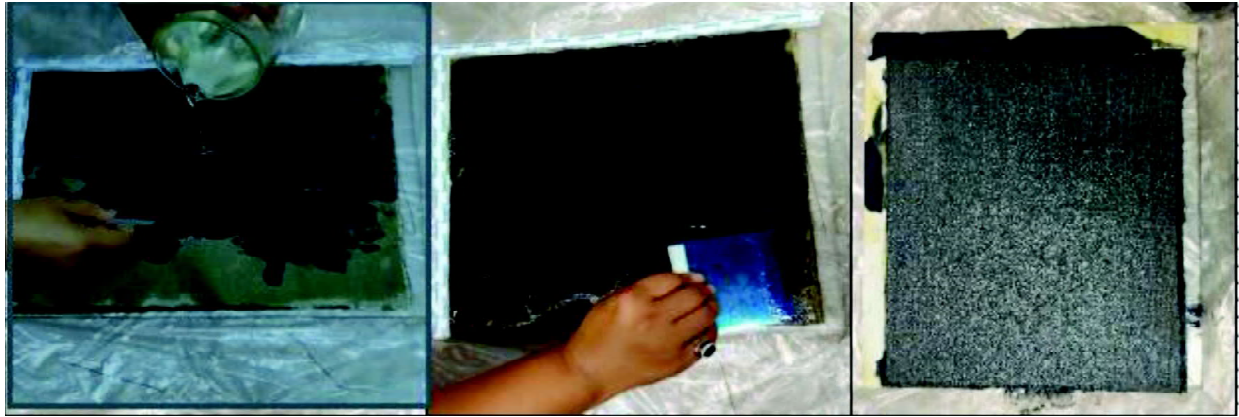
Fig.8: Spreading the resin-filler mixture onto the fiber mat during lamination
