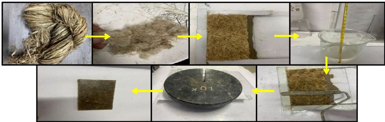
Fig. 6: Step-wise Epoxy based Hand Lay-Up casting process
