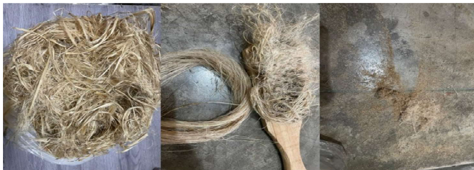
Fig. 2: Chemical-free surface cleaning of Grewia optiva reinforcement via manual combing for enhanced interfacial bonding
