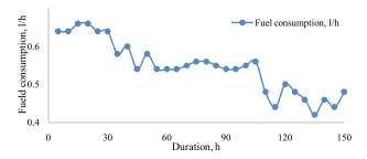
Fig. 3: Fuel consumption of engine during the long duration test Exhaust emission
