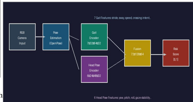
Fig. 3: Gait and Head Pose Feature Extraction Pipeline - dual-encoder behavioral signal processing
